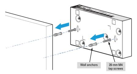
3. For under-table mounting, a third 20-mm M4 tap screw can be placed against one side of the switch to secure it in place.
