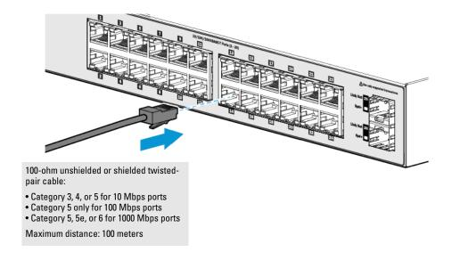
When a network cable from an active network device is connected to the port, the port LEDs for that port should go on. If the port LEDs do *not* go on when the network cable is connected to the port, see "Diagnosing with the LEDs" on page 4-2.
