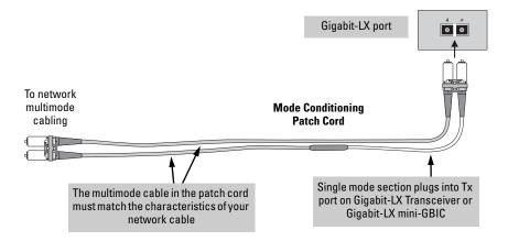
**Example: Connecting a Mode Conditioning Patch Cord for Gigabit-LX**
